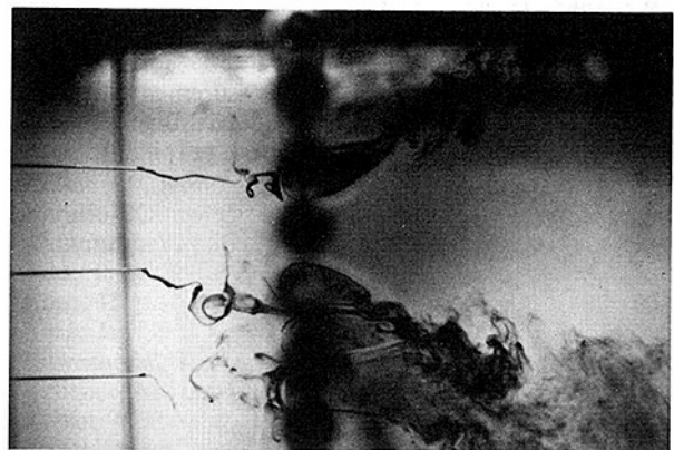
Fig. 1 Visualization of water flow through a tightly spaced row of tubes. The jets emerging between the tubes deflect sharply and join into groups at the top and bottom of the picture, leaving a stagnant zone in the center. Similar observations were made after double (in-line) tube rows.
